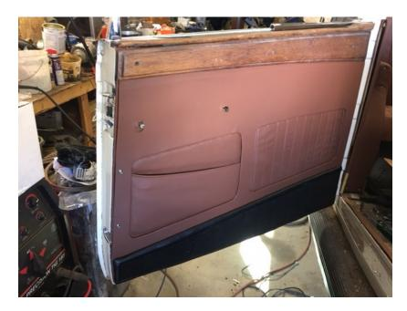
The panels on the doors and rear areas were thin plywood. In the proper British tradition, the panels that were on the car had been host to several insect species. I was able to hold them together just long enough trace around them for new panels made from one quarter Baltic Birch and dismantle the fabric for clues on how they were put together. Clues for the Clueless.
