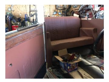
put the fabric over the padding and sew straight through or you can layout the pleats then fold the fabric back on itself and sew through the edge that is presented. The first is pretty straight forward and shows the stitching. The second hides the stitching. Apparently, this gives a directional bias to the tuck and roll that favors one direction over the other as you
