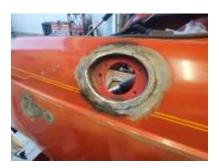
Repositioned the gas fill to the right rear quarter and filled the old filler spot.
