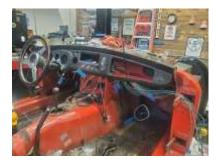
3) Removed and replaced the dash scuttle with a Heritage piece that will allow me to use an older metal dash rather than the pad-
