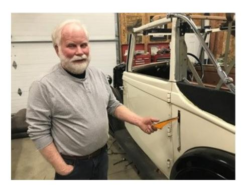
Turn signals. Standard had turn signals in 1936. What next? Perhaps a heater would be nice. The original turn signals were an electric type of semaphore. Selecting a turn would energize an electromagnet that pulled a flag out of a slot and turned-on lights inside the attached housing. It was a steady light and not
